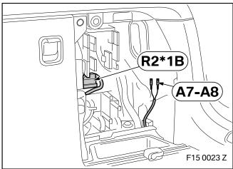
Connect branches **A7–A8** as follows to plug **R2\*1B** SW 24-pin socket casing:
