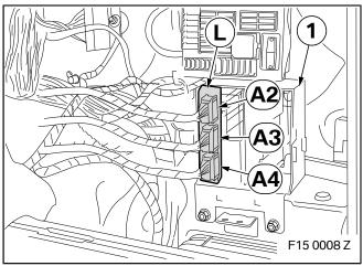
Insert AAG control unit  ${\bf L}$  in the control unit holder (1).
