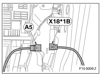
Connect branch **A5**, SW 3-pin socket casing, to plug **X18\*1B**, SW 3-pin pin housing.
