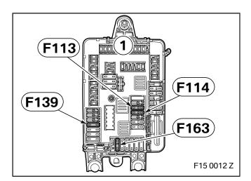
Check that 30 A fuses are inserted into slots **F113**, **F114**, **F163** and a 20 A fuse is inserted into slot **F139** of the rear right fuse box (1).
