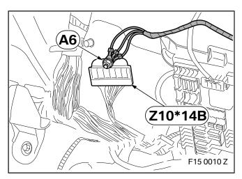
Screw branch **A6**, M6 ring eyelet, onto ground support point **Z10\*14B**.
